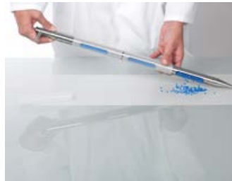
Sealing sleeves zone sampler 25 mm usage
